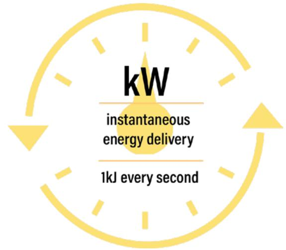
*Think of kilowatts (kW) like the rate at which water flows in to a glass. Think of kilowatt-hours (kWh) like the total amount of water in that glass.*
