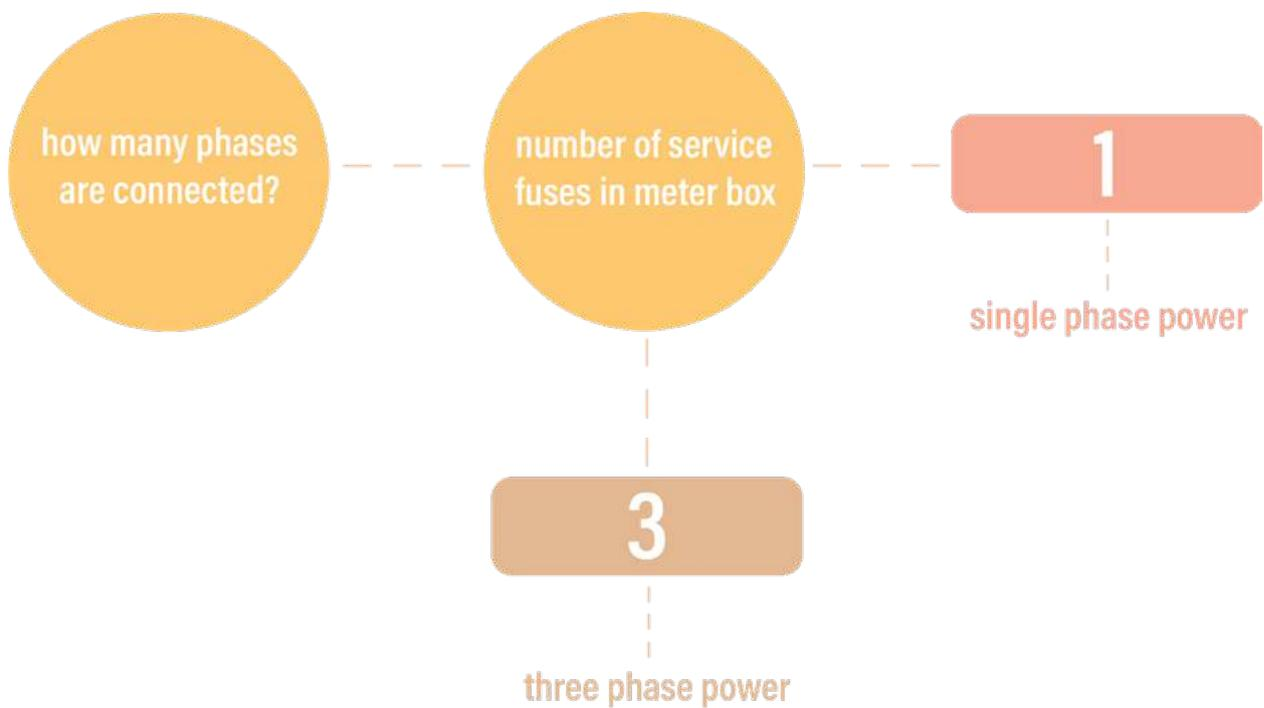
You can tell how many phases you have by the number of service fuses in your meter box (make sure it's the main one and not a distribution board or sub board).
